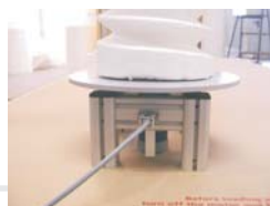
Milling axis 200W with mounts for hand milling machine and shaped wire lance
